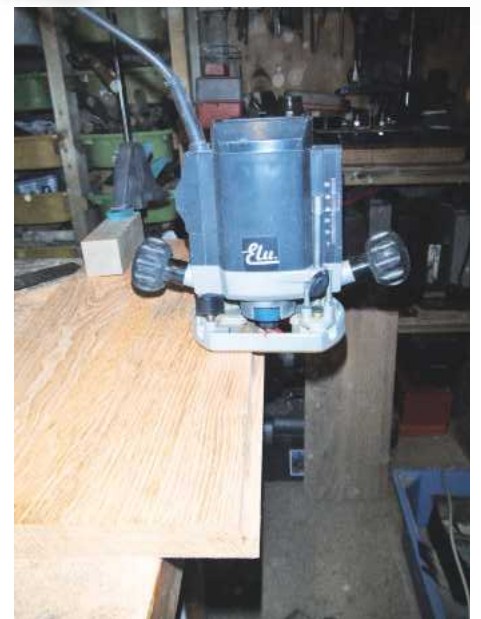
▲ Pic.4 Edge routing the table flaps
